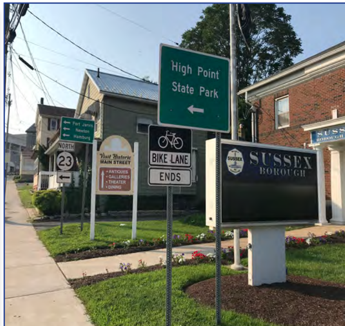
Images 79 and 80. Sign clutter in the median at the intersection of Hamburg Avenue (State Route 23 northbound) and Main Street (left) and in front of Sussex Borough Hall (right). NJDOT signs leading to points outside of the Borough overwhelm the “Visit Historic Main Street” and “Shop Small Sussex” signs and encourage drivers to stay on the curve to follow State Route 23 instead of travelling straight onto Main Street.
